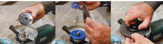
**ASSEMBLY: VIBLOCK** is quick and easy to assemble.
